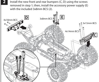
Important Note! Use the included power tap as the direct battery source for the accessory power supply. Do not connect to the accessory BEC power output on the ESC (if equipped). Connecting high-load accessories to the power supply while it is plugged directly into the ESC could overload the speed control's BEC circuit. This may cause the speed control to go into thermal protection mode or could cause damage to the speed control.
